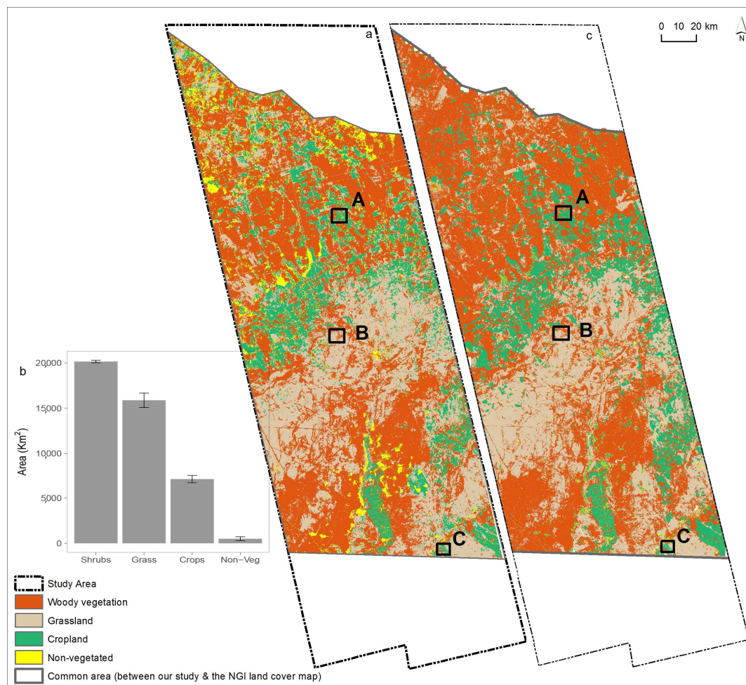
Figure 5. (a) Land cover map from the best performing model of this study (Model#9 in Table 3); (b) error-adjusted area estimates and 95% confidence interval margins for the four land cover classes estimated from the best performing model; and (c) the 2010 high resolution (SPOT 5 and colour infrared aerial photography-based) land cover data of the South African National Geospatial Information (NGI) mapping agency [43]. Locations A, B and C are the example subsets that appear in Figure 7.
