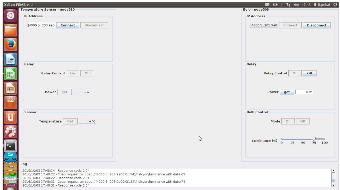
Figure 4.5: Constrained Application Protocol (CoAP) interface showing the monitoring (sensor) and control (lamp) windows.
