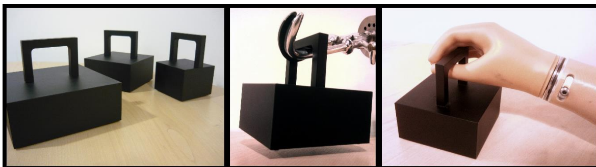
Figure 1. One set of the small, medium, and large objects used in Experiment 1, as well as examples of how the objects were lifted with different types of prostheses.
