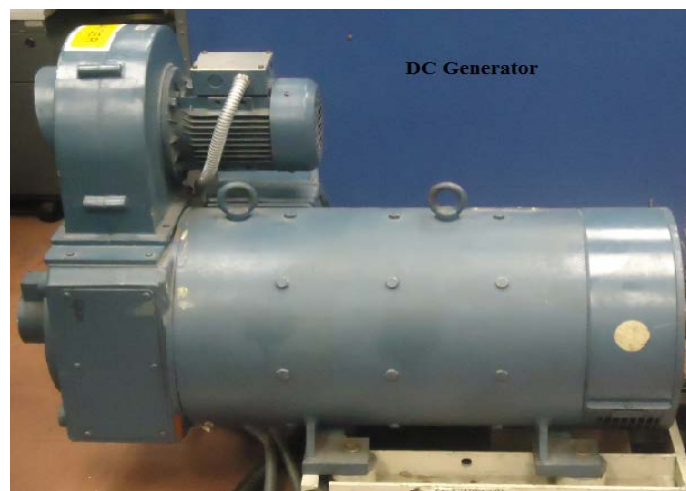
Figure6.6 DC generator (mechanical load)
