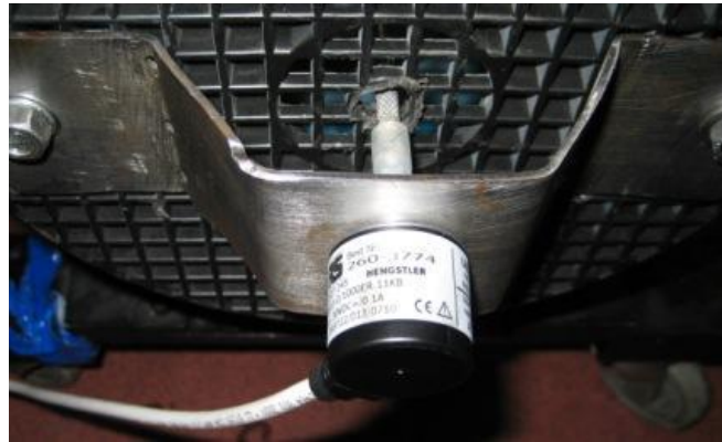
Figure 6.11 Mounting of motor encoder
