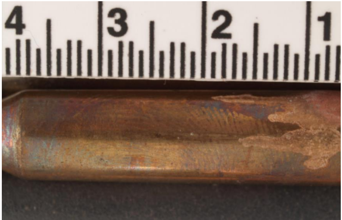
Figure 1-4 Electrolysis-etched fingerprint on a bullet. Reproduced from Reference 30 with permission from the International Association for Identification.
