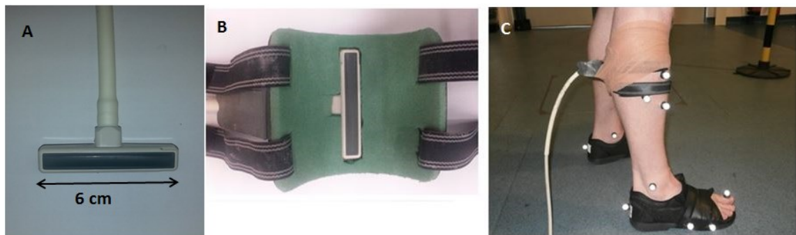
Figure 1. A linear 7.5 MHz probe (A) with 60 mm field of view. A custom-built fixation device made of Velcro straps and a plastic cast molded to fit the general contour of the calf (B) was used to secure the probe around the left lower leg, in the mid-sagittal plane of the gastrocnemius muscle (C) (Fukunaga et al., 2001).
