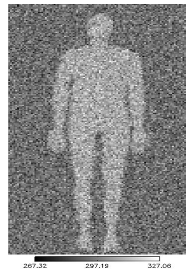
Figure 5: Scene simulation [2] of a person against an absorber background indoors when the system sensitivity is close to the subject background contrast.
