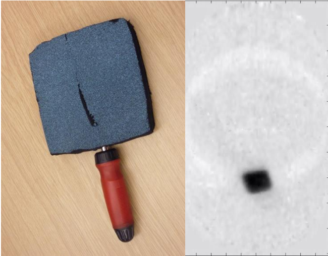
Figure 4: A 16cm square section of absorber (left) is dipped in liquid nitrogen and physically moved from the bottom to top in the FOV at the nominal range of 1.6 m to absolutely calibrate all receiver channels, a snap shot image through this process is shown (right).
