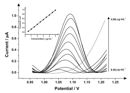
Fig. 3 Differential pulse voltammograms of the screen-printed graphite electrode by adding aliquots of PMA (in phosphate buffer pH 7.0) at concentrations in the range of  $0.50-4.98~\mu g~mL^{-1}$  (in phosphate buffer supporting electrolyte); the dotted line represents a blank. (inset) An analytical curve corresponding to the anodic peak for the oxidation of PMA over the concentration range (E-step: 0.002 V; E-pulse: 0.1 V; tpulse: 0.05 s; scan rate: 0.005 V s<sup>-1</sup>; t-eq. 1 s)
