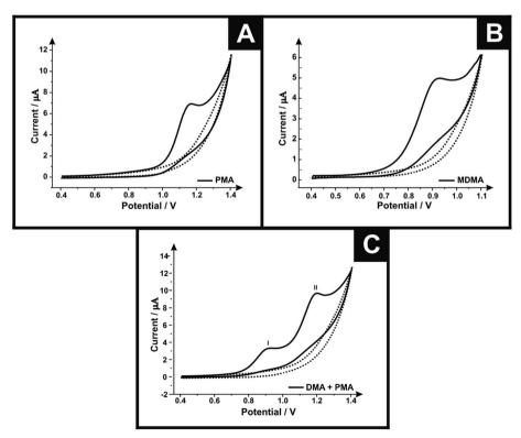
Fig. 1 Cyclic voltammograms of SPE (A) in presence (500  $\mu g$  mL<sup>-1</sup>) and absence of PMA, (B) in presence (250  $\mu g$  mL<sup>-1</sup>) and absence of MDMA and (C) in presence (250  $\mu$ g mL<sup>-1</sup>)/(500  $\mu$ g mL<sup>-1</sup>) and absence of MDMA/PMA in PBS (pH 7) (scan rate: 100 mV s<sup>-1</sup>).
