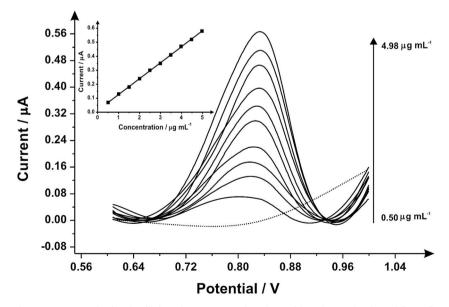
Fig. 2 Differential pulse voltammograms obtained utilizing the screen-printed graphite electrodes by adding aliquots of MDMA (pH 7.0) at concentrations in the range of  $0.50-4.98~\mu g~mL^{-1}$  (in phosphate buffer supporting electrolyte); the dotted line represents a blank. (inset) An analytical curve corresponding to the anodic peak for the oxidation of MDMA over the concentration range (*E*-step: 0.002~V; *E*-pulse: 0.1~V; *t*-pulse: 0.05~V s<sup>-1</sup>; *t*-eq. 1 s).
