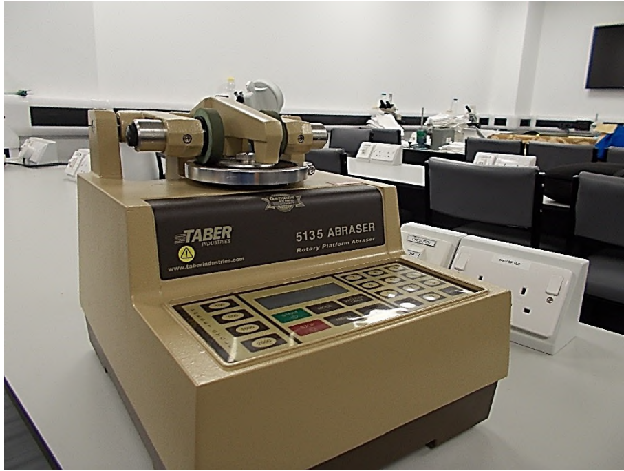
Figure 7 Taber Abrasion Tester
