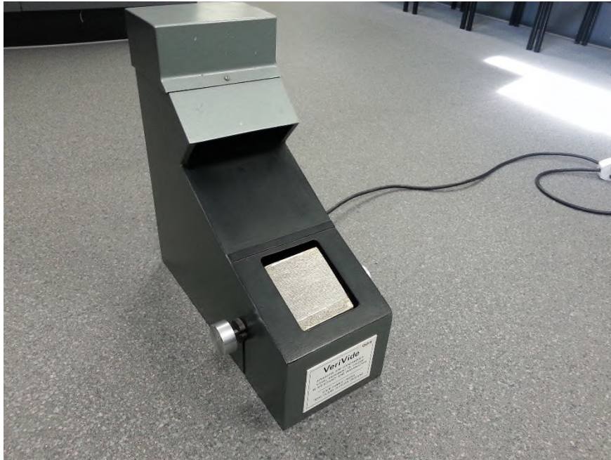
Figure 12 Pilling assessment photographs
