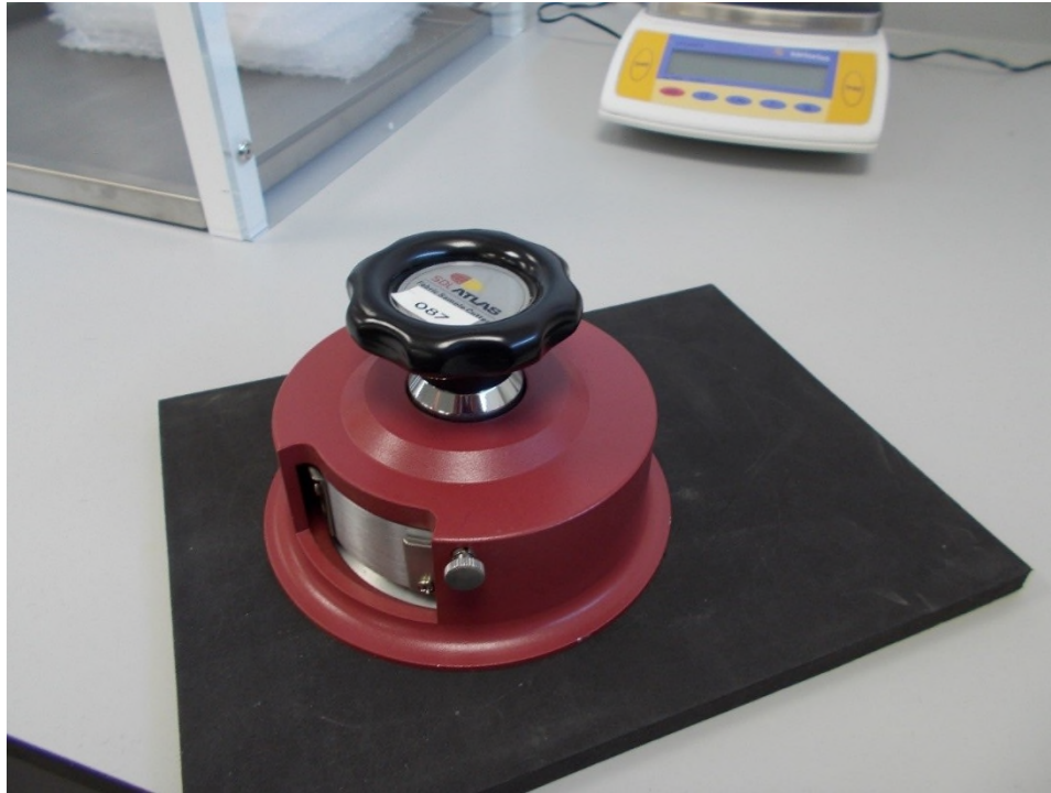
Figure 2 Fabric gsm cutter (Image courtesy of MMU Textile Lab)
