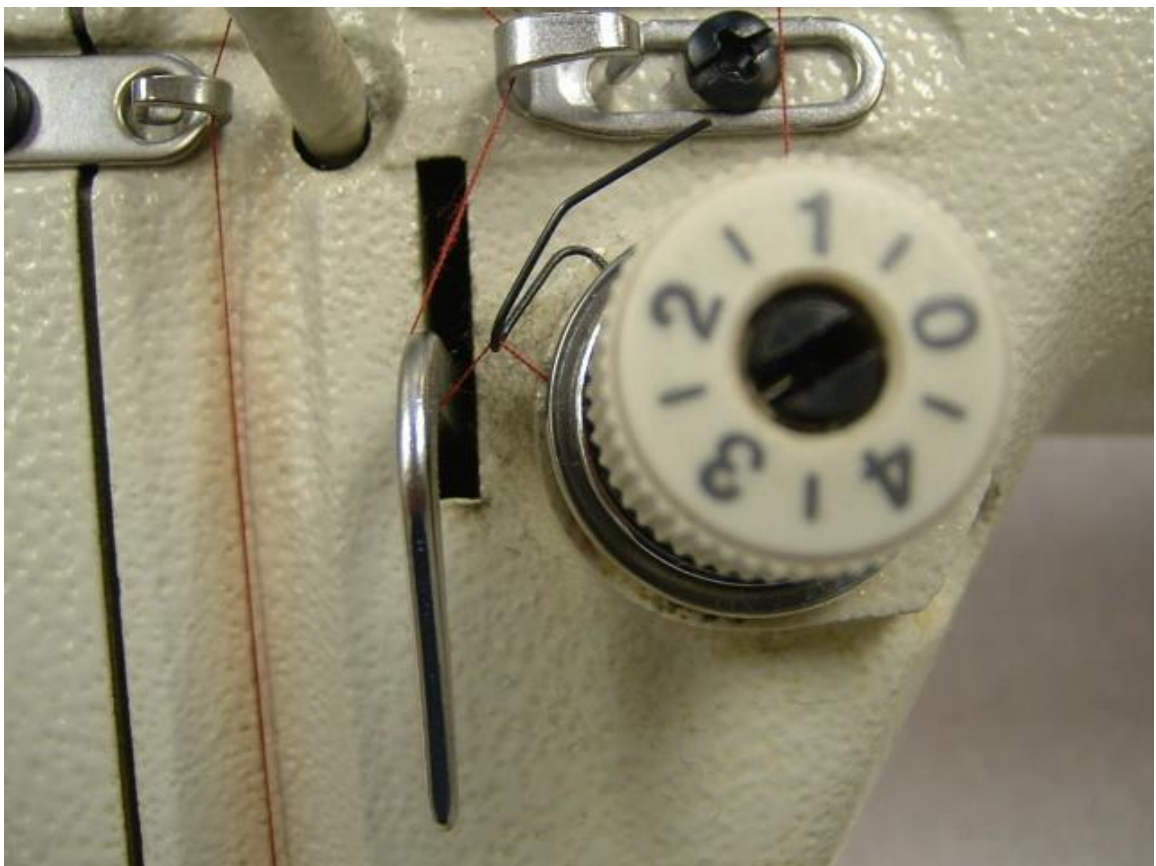
Figure 3.18: Check spring (2) should wink (move) when thread is at the Six O -Clock position
