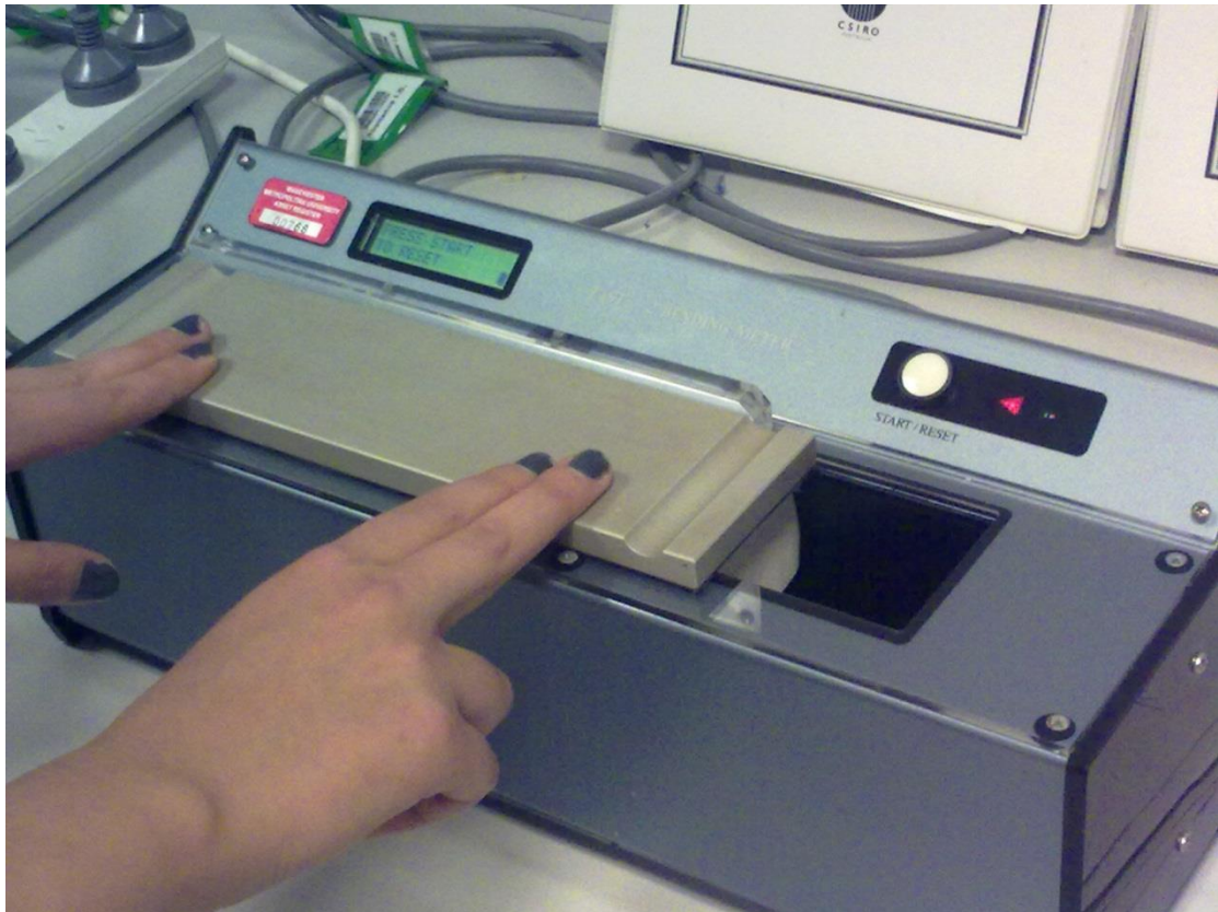
Figure 5.4: FAST 2 – Bending stiffness tester
