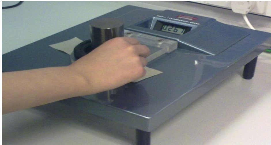
Figure 5.2: FAST-1 – Surface thickness tester measurement testing device
