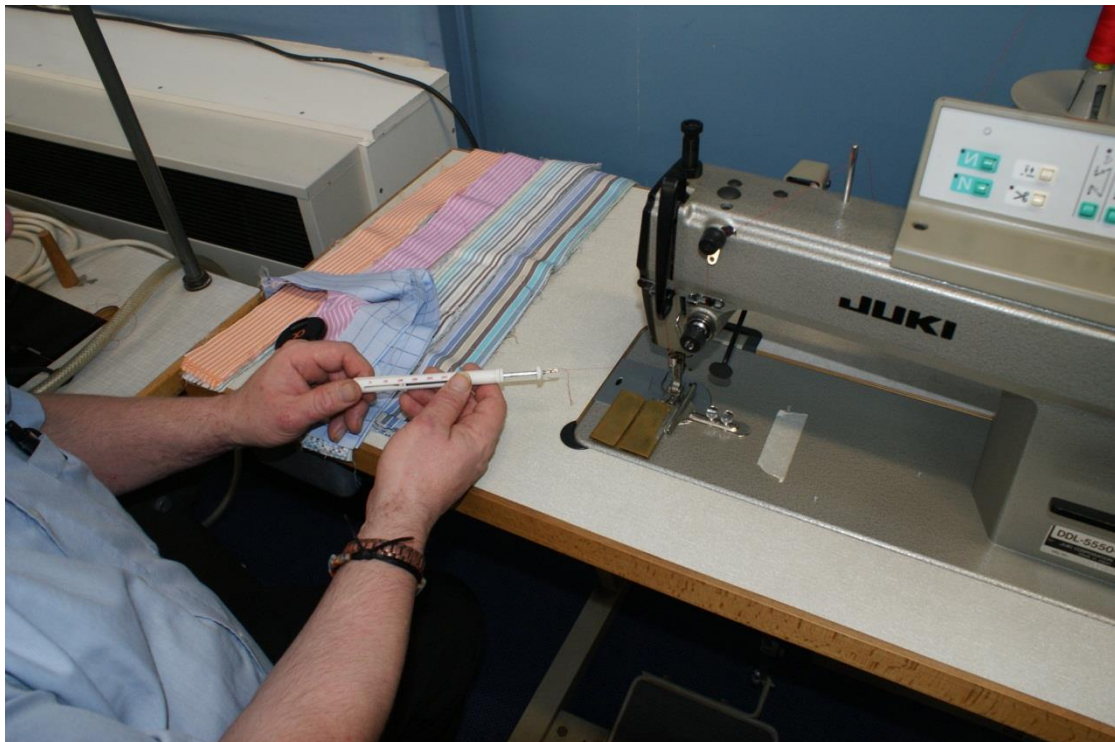
Figure 5.27: Pencil sewing thread tension measurement device
