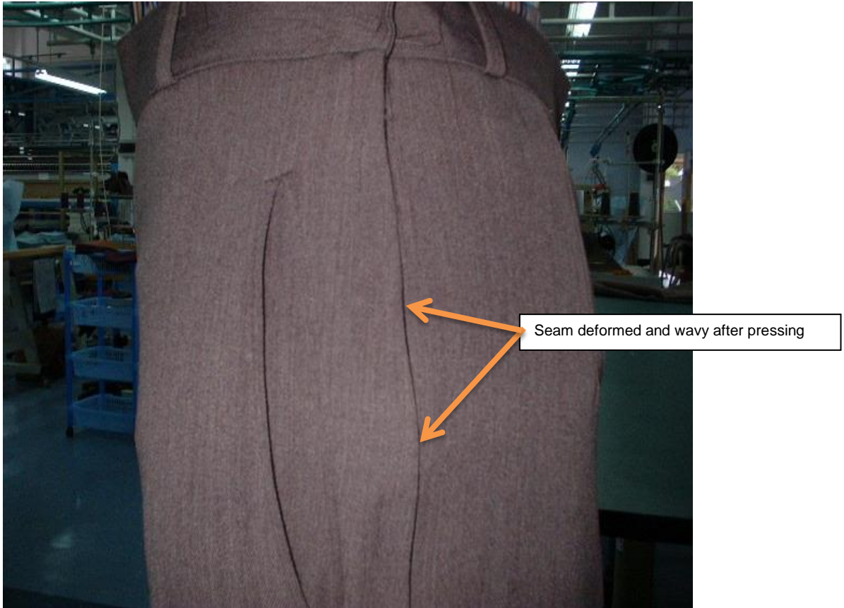
Figure 3.9: Feed pucker on the zip after pressing
