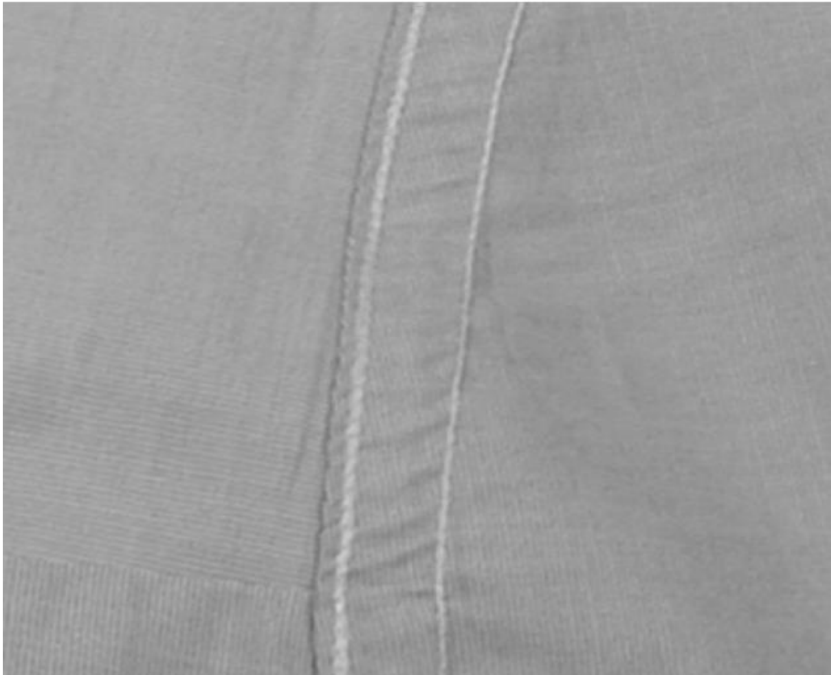
Figure 2.13: Feed puckering holding back the upper ply
