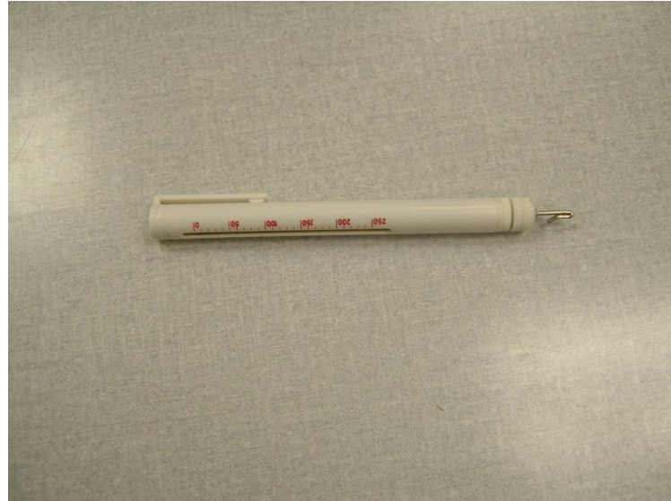
Figure 6.5: Tajima pencil thread measurement gauge
