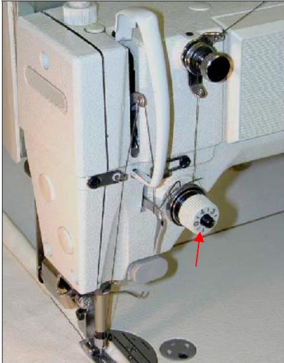
Figure 2.12: Excessive thread tension
