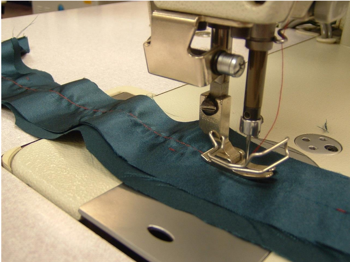
Figure 1.1: Example of seam pucker on two plies of fabric
