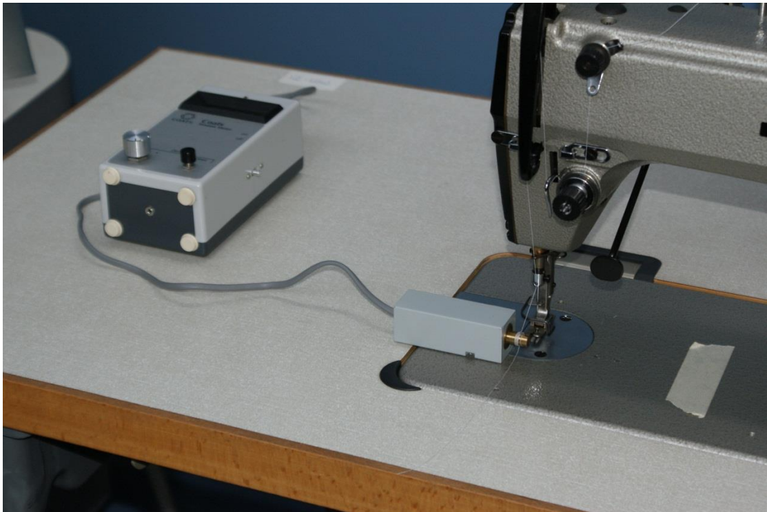
Figure 3.4: COATS thread tension metering device
