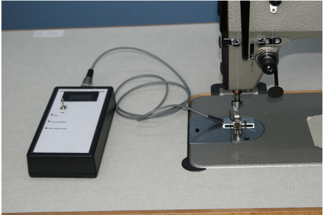
Figure 6.7: Presser foot pressure measured electronically
