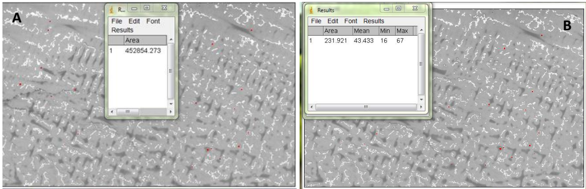
Figure 3-9 Surface area of the scanned area (A), surface area of pores (B)
