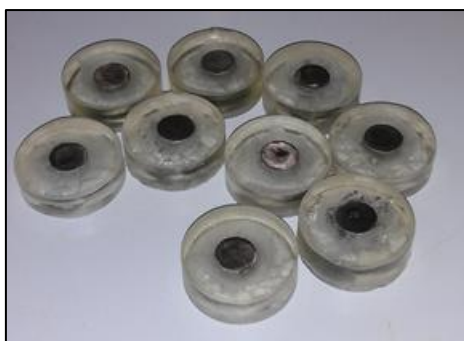
Figure 6-1 Test pieces embedded in mounting resin
