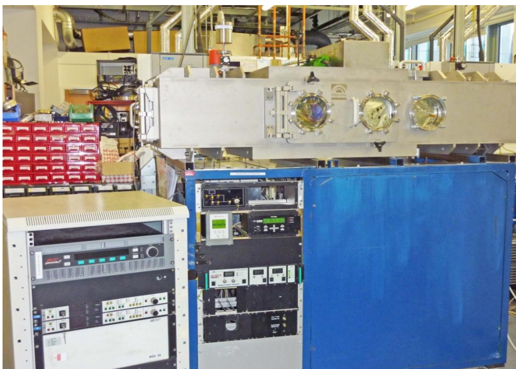
Figure 7.1: Large Area coating chamber (Prevac Sp. z.o.o.)
