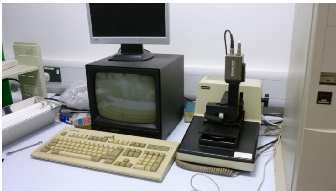
Figure 8.1: Picture represents Dektak 3 stylus profilometer used to physically measure coating thickness after deposition.
