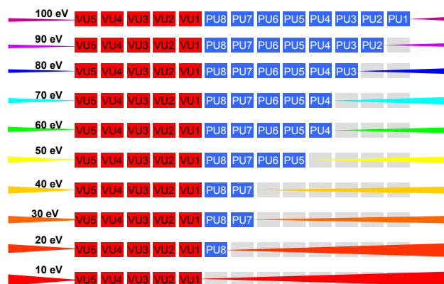
Figure 10. Schematic of the modular undulator system and focusing lattice of the XUV-FEL demonstrating the different modes of operation across the photon energy range 10–100 eV. Electron beam transport and seed injection is right to left with increasing z . Undulator modules marked in grey have large magnetic gaps \bar{a}_u \approx 0 and are effectively absent for the purposes of the FEL interaction. The minimum required undulator gap (and vacuum vessel internal aperture) decrease in gradual steps from 28 mm (25 mm) for PU1 down to 10 mm (7 mm) for PU8 and the variable polarisation modules VU1..VU5. Radiation beam waists of the seed and output are shown from 100 eV (violet) to 10 eV (red).
