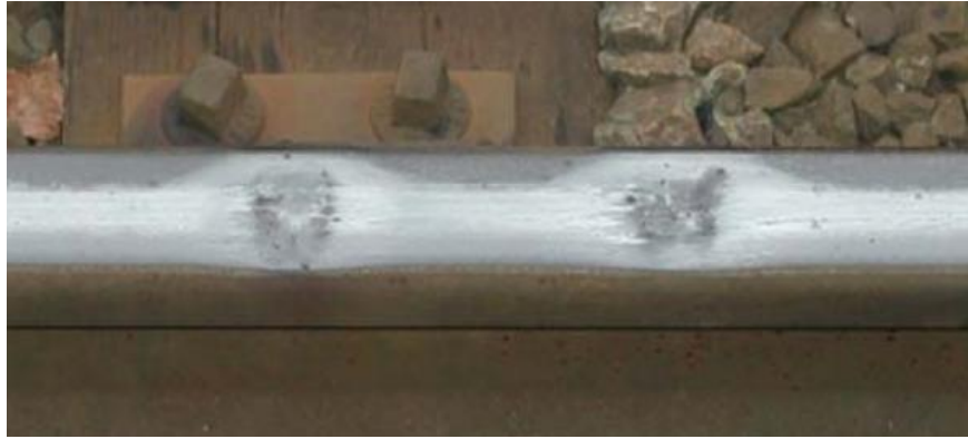
Figure 5.47 A photograph of wheel burns on the running surface of flat bottom rail.
