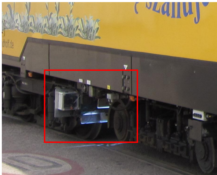
Figure 4.16 Photograph of the Tri-linear LED design implemented and mounted on Warsaw Tramway (Tramwaje Warszaws) vehicle.
