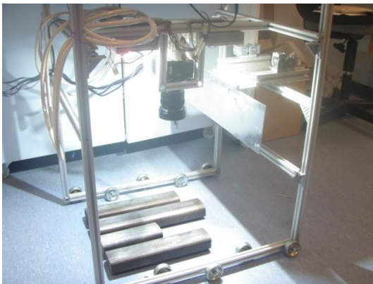
Figure 4.5 Photographs of light testing on low speed trolley for lab based image acquisition of rail.
