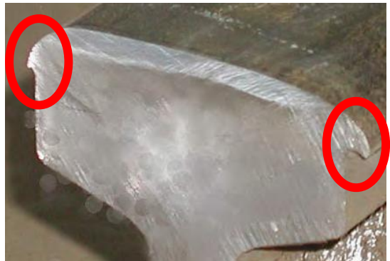
Figure 5.43 A photograph of a cut piece of rail with plastic deformation
