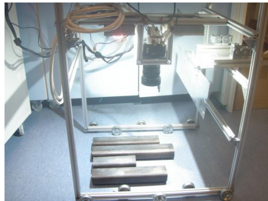
Figure 4.5 Photographs of light testing on low speed trolley for lab based image acquisition of rail.
