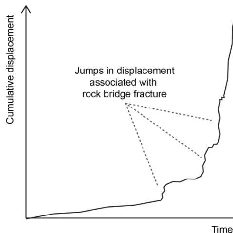
Figure 2.6: Schematic of cumulative displacement observed for failure of brittle slope failures and rockfalls. Steps or jumps in the cumulative displacement may be related to rock bridge fracture events (Carlà et al., 2017; Kromer et al., 2015; Royan et al., 2015).
