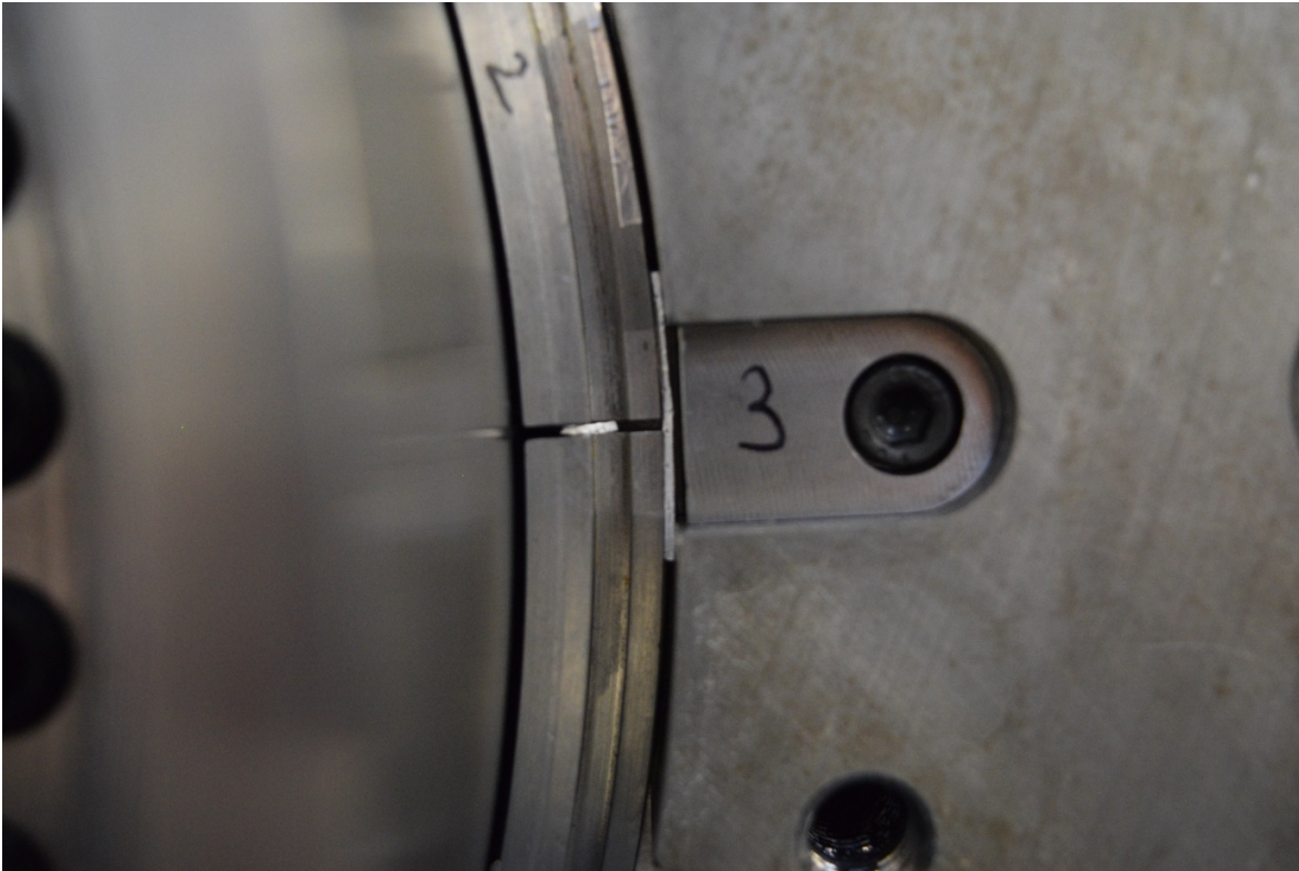
Figure 6.15: Seal segments fixed into position with aluminium shims.
