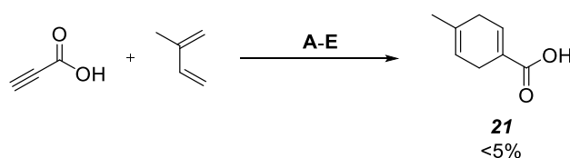
Scheme 4.2 Alternative reaction conditions to synthesise 19 . (A) CH 2 Cl 2 , rt, 16 h; (B) Hydroquinone, toluene, 120 °C; 195 (C) Sealed vessel, toluene, 120 °C; (D) CuI, Et 3 N, CH 2 Cl 2 , rt; 196 (E) AlCl 3 , CH 2 Cl 2 , 40 °C. 197
