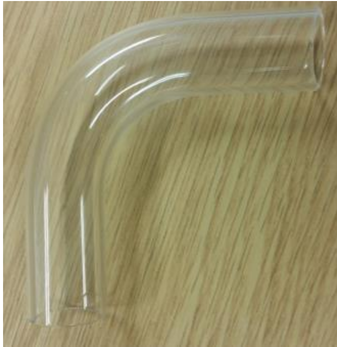
Figure 66: The custom built glass tubing, approximate 90 mm x 90 mm. The glass tube was dried in between each sample
