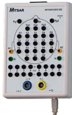
Figure 6.3.7.2: Mitsar 202 EEG amplifier.
