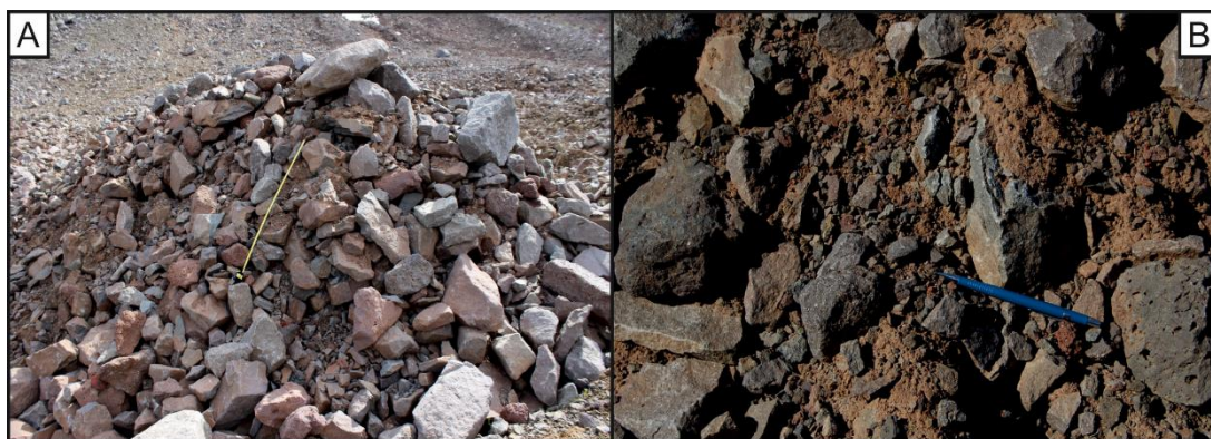
Figure 6.3. Material comprising molards. (A) A molard in Móafellshyrna showing coarse deposits on the surface with no gradation. (B) Typical internal granulometry of a molard, composed of unsorted gravel in sandy silt to silty clay matrix.
