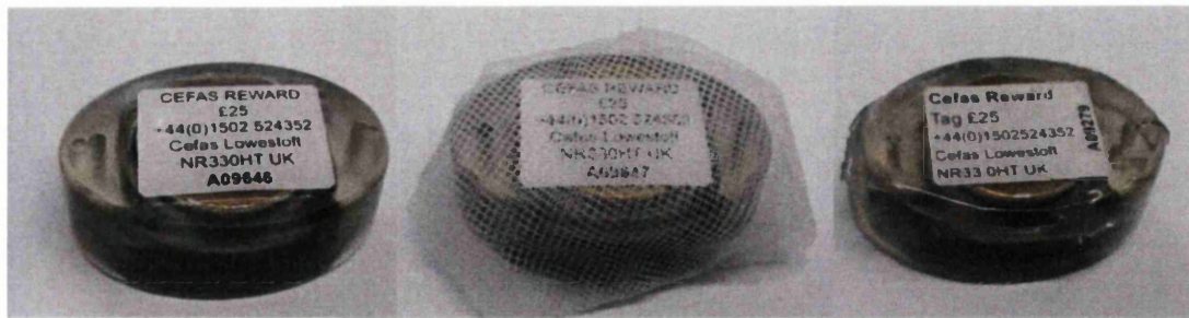
Figure 2.1. CTL (Cefas Technology Limited) G6a tags (a) uncoated, (b) coated in surgical mesh and (c) coated in medical-grade silicone.
