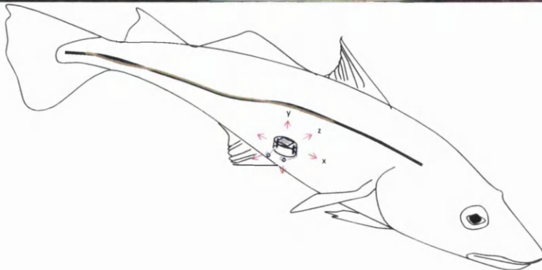
Figure 1.2. Tri-axial accelerometer in the body cavity of an Atlantic cod ( Gadus morhua ), showing the surge (x), heave (y) and sway (z) axes of motion.
