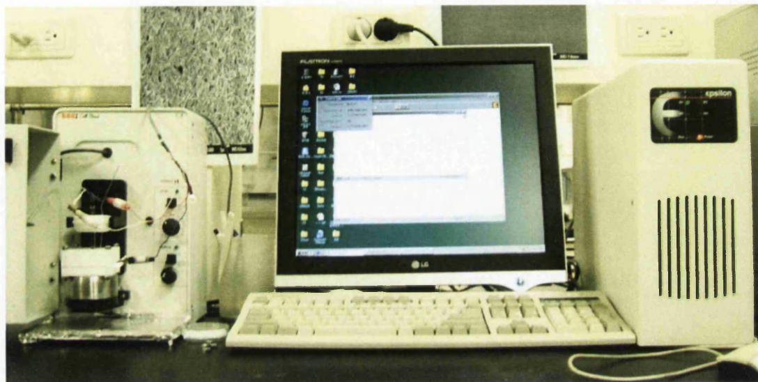
Figure 3-6: Polarographic system for zinc concentration measurement
