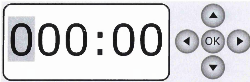
Figure 4.1: An example of 5-key user interface layout. Here the cursor is shown in the left-most position, and the display format is suitable for entering times, 0 minutes to 999:59 hours. Some 5-key interfaces omit the OK button as its use can be implied by the user performing any action with any non-arrow button.
