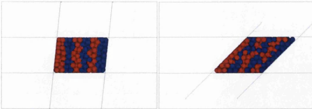
Figure 5.2: The method of shear induction in the small scale percolation tests [105]. The strain rate was governed by the period of the angular deformation.
