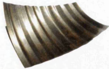
(b) Twisted bi-stable corrugated core (Norman et al., 2007)
