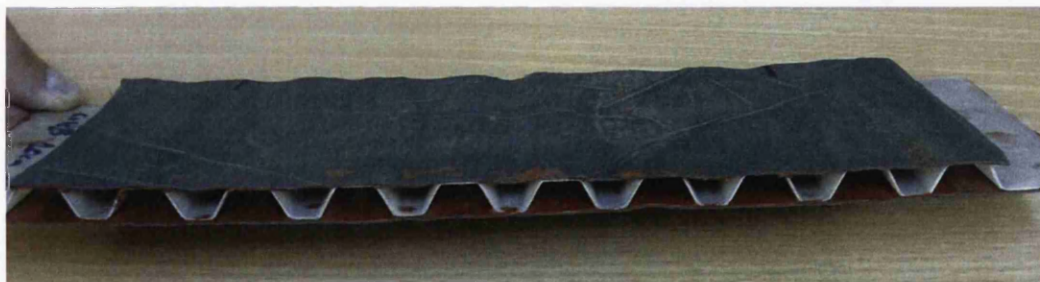
Figure 2-7: The coated composite corrugated core, (Dayyani et al., 2013)
