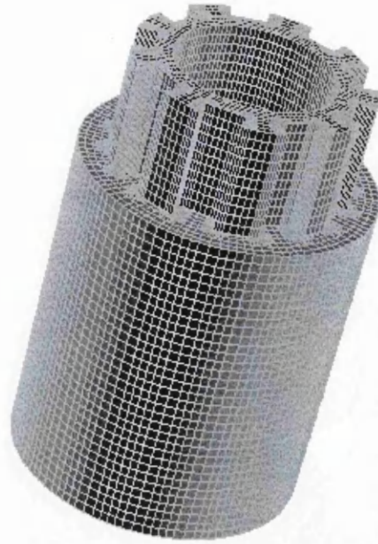
Figure 7 Multiblock mesh example
