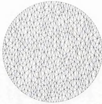
Figure 22 Mesh resulting from anisotropic metric
