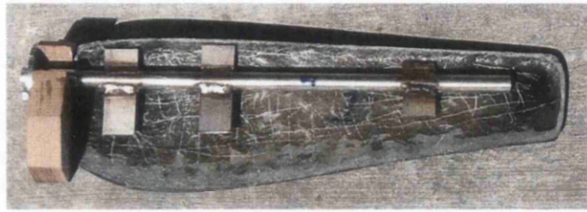
Figure 3.14 - Stainless spar inserted and aligned in finished blade half
