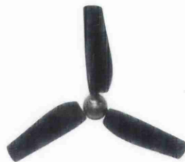
Figure 3.15 - Finished rotor blades on 3 bladed hub.
