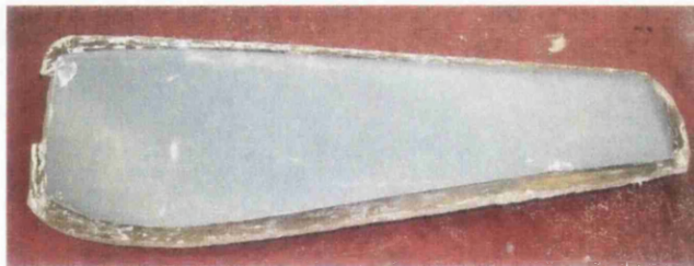
Figure 3.13 - The blade plug in one half of the mould
