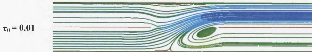
Figure 5.18: (a) Streamline patterns: Herschel-Bulkley fluids, Re=50 , m=0.6 , k=1.0
