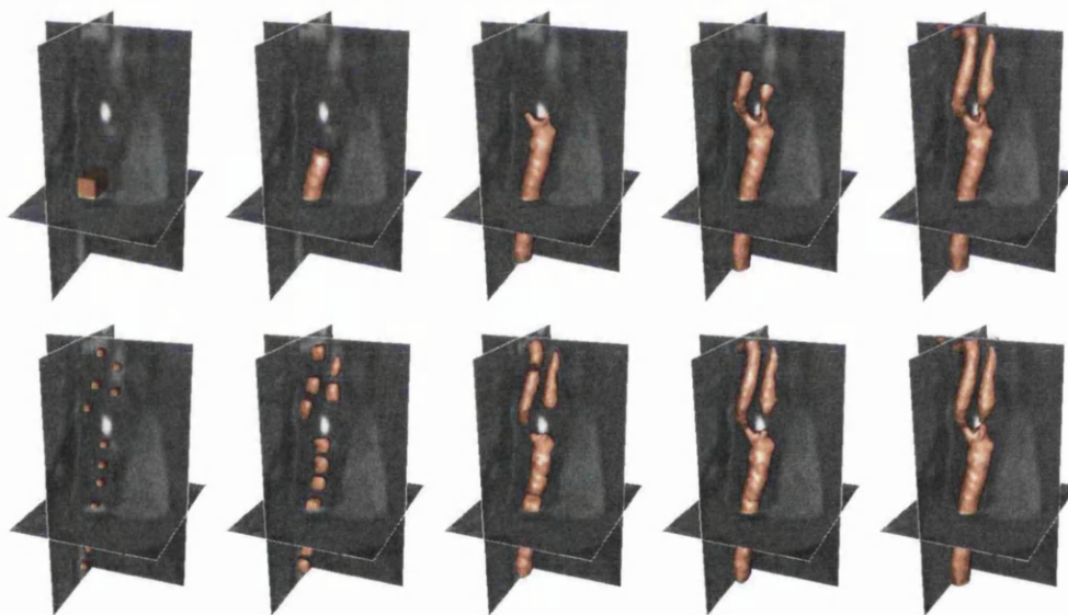
Figure 4.7: Segmentation of carotid artery from CT image dataset 3 ( 70 \times 80 \times 120 ) using GPF deformable model with different initializations (top row: CPU-time, 979s, bottom row: CPU-time, 206s).
