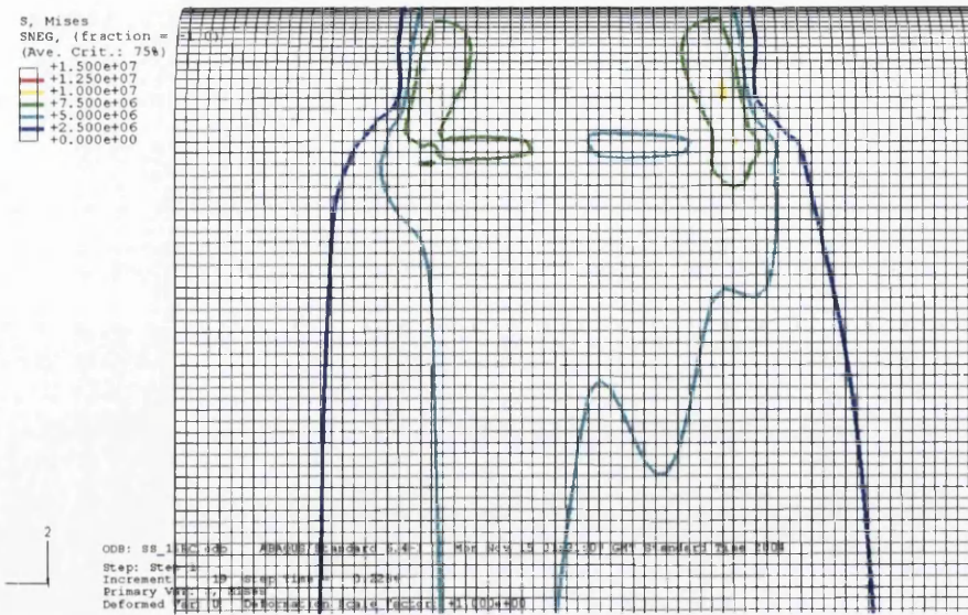
Figure 7.18 Model 2.11 - von Mises equivalent stress - Tension 3MPa
