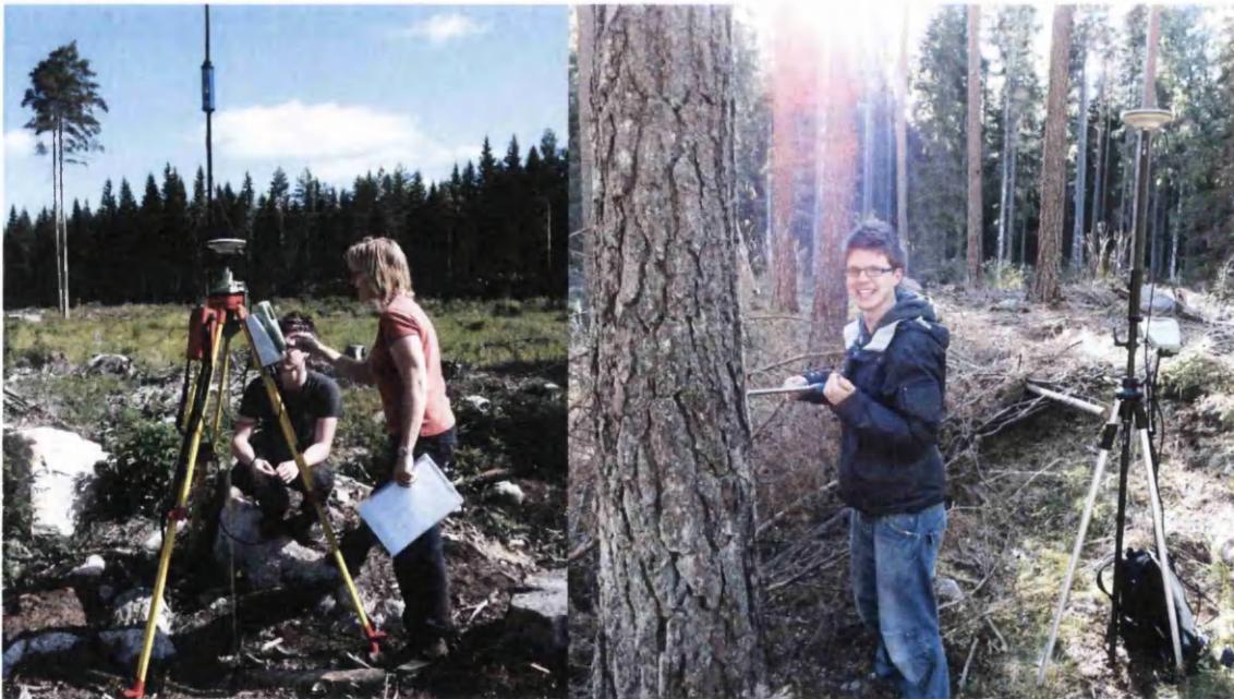
Figure 3.6: Leica GX1230 GPS base system while Natascha Kljun and Craig Mahoney are operating it (left). Leica GX1230 GPS Rover taking the tree position relative to the base while Craig Mahoney is taking a core from a tree (right).
