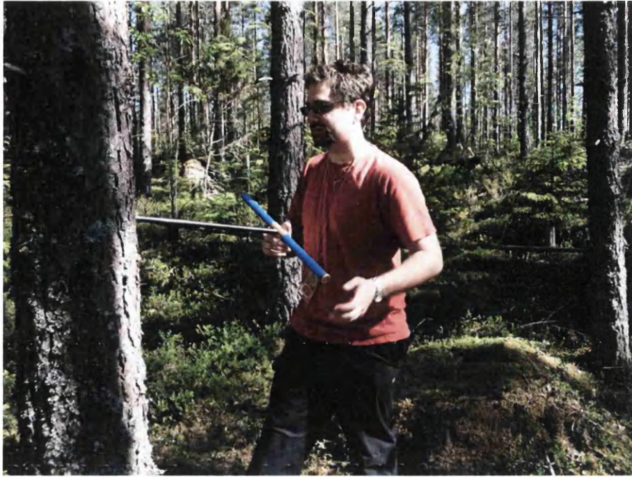
Figure 3.5: Coring process on a Scots pine tree by using a 12 mm borer in Finland.
