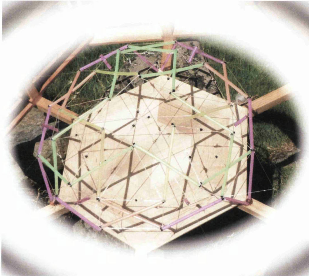
Figure 2.17: Deployable, geodesic tensegrity dome model, mounted in a hexagonal box.
