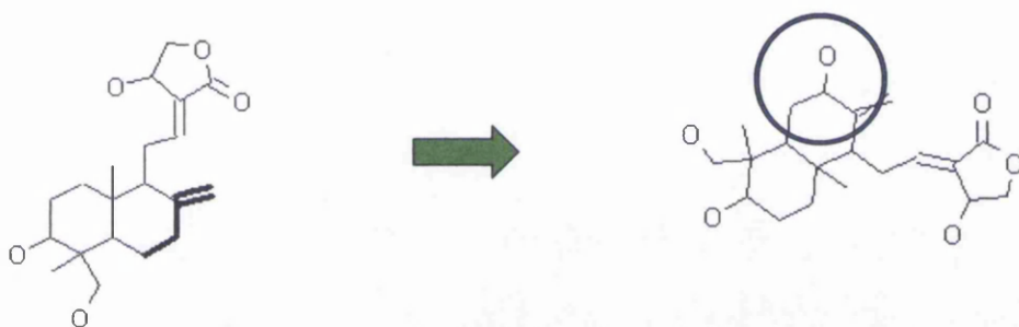
Fig. 2.16e. Allylic hydroxylation. Area in bold print is the reaction substrate whereas the blue ring denotes structural transformation.
