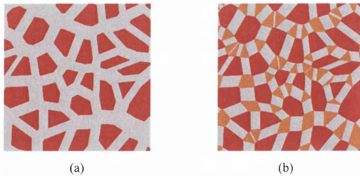
Figure 7.2.8 (a) Synthetically developed microstructural model for NPC material based on the modified double line Voronoi (i.e. this double line area is considered as microstructural Ig phase in the model) (b) Synthetic microstructural model based on modified three phase microstructural model (i.e. the double line Ig phase is divided into two regions as GBAZ and TJ with sharp corners).
