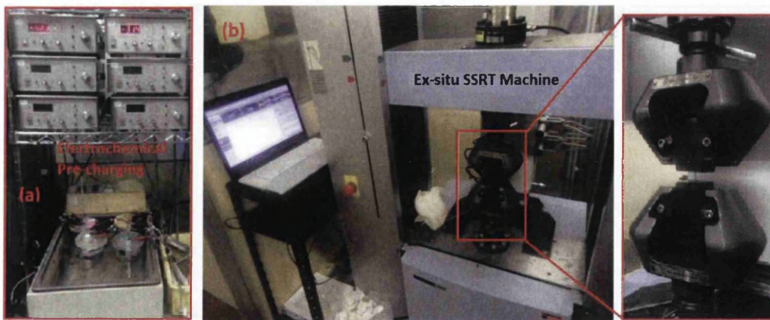
Figure 4.4.2 (a) shows the electrochemical charging cells and (b) shows the ex-situ SSRT testing machine.
