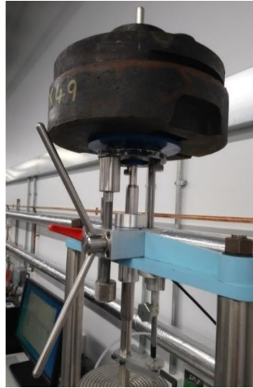
Figure 4. Capstan style load release mechanism.
