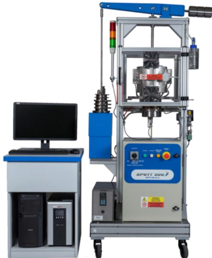
Figure 1. SPUTT 500 - Small punch creep testing machine.
