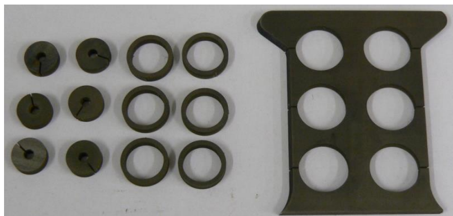
Figure 9. Ring specimens and remains from EDM operations.
