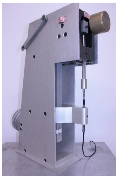
Figure 2. LVDT interfaced to a certificated calibration rig.
