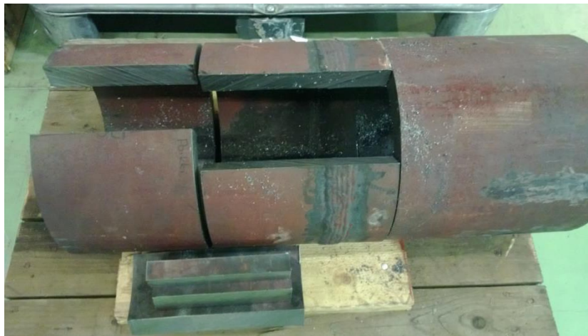
Figure 1. Welded 10CrMo910 pipe (273*32mm) after removal of test specimens.
