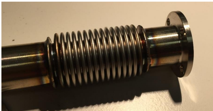
Figure 5. Metallic bellow welded into a stainless tube.
