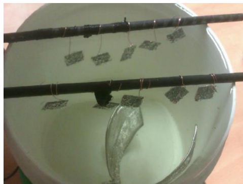
Figure 8. SPT pre-embrittled specimens during its hydrogen absorption.
