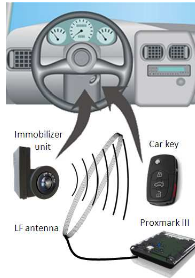
Figure 5: Experimental setup for eavesdropping
