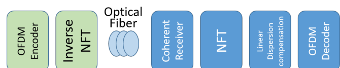
Fig. 1. Basic elements of the communication system based on the nonlinear inverse synthesis.
