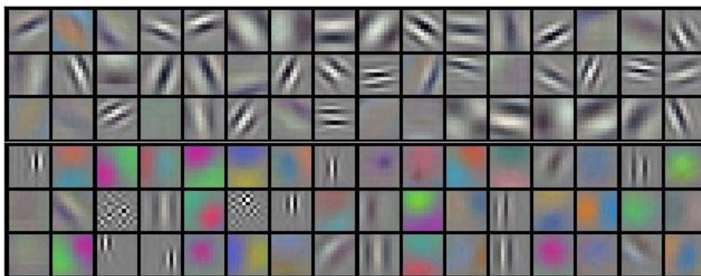
Figure 2. The convolutional filters from the first layer of the Alexnet neural network (Krizhevsky et al., 2012). Each filter is 11 by 11 pixels. The neural net was implemented on 2 GPUs, which did not communicate until higher layers. (A GPU is a graphics processing unit and is frequently used to speed neural net training.) The top 48 filters are from GPU1 and the bottom 48 from GPU2. The filters on one GPU tend to specialize in encoding luminance changes, and the filters on the other GPU tend to specialize in color. Reprinted with permission from Krizhevsky, A., Sutskever, I., & Hinton, G. E. (2012). ImageNet Classification with Deep Convolutional Neural Networks. In F. Pereira, C. J. C. Burges, L. Bottou, & K. Q. Weinberger (Eds.), Advances in Neural Information Processing Systems 25 (pp. 1097–1105). Curran Associates, Inc.
