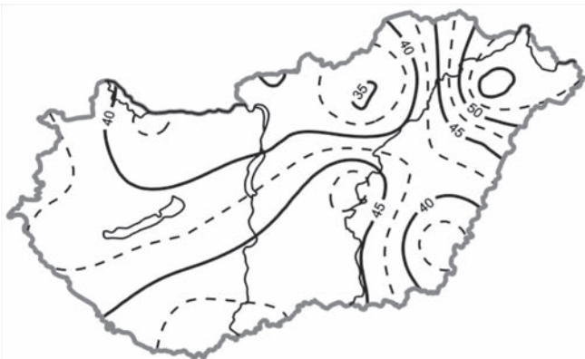
Figure 6 – The mean values of coefficients of variation (CV) of the absolute daily maxima of precipitation in spring measured at 16 stations over a period of 1951–2010
