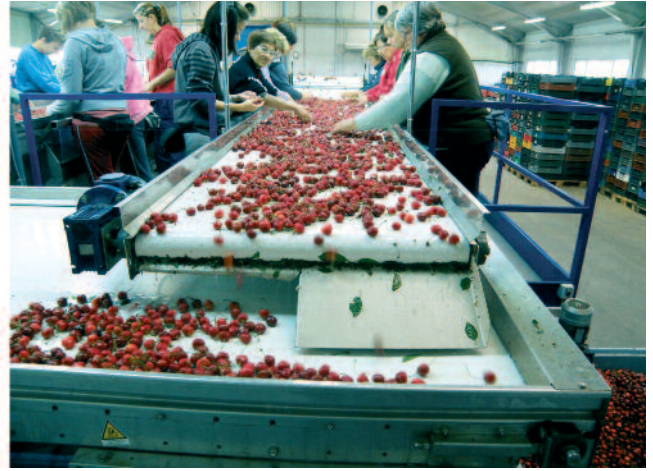
Fig. 4: Longitudinal sorting belts
