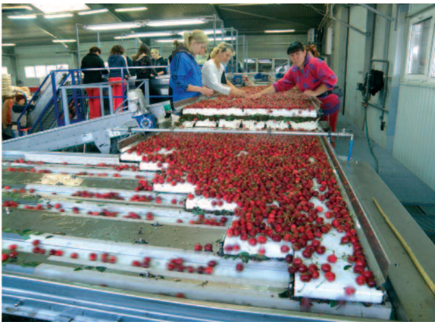
Fig. 5: Transverse collecting belt
