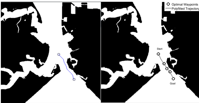
Fig. 3. Generated (left) and smoothed trajectory (right) from the optimal waypoints produced by the path planner. Binary map of 800 x 800 resolution is considered for the current study with one pixel representing 3.6 m on a real map
