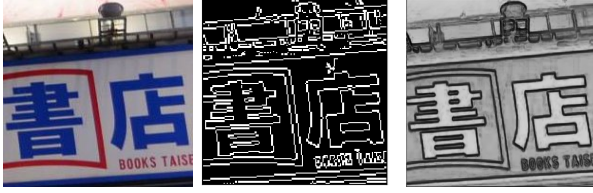
Figure 3. Comparison of edge detection for Canny and HED. Left to Right - Image, edge output of Canny, edge output of HED. Best viewed in pdf.
