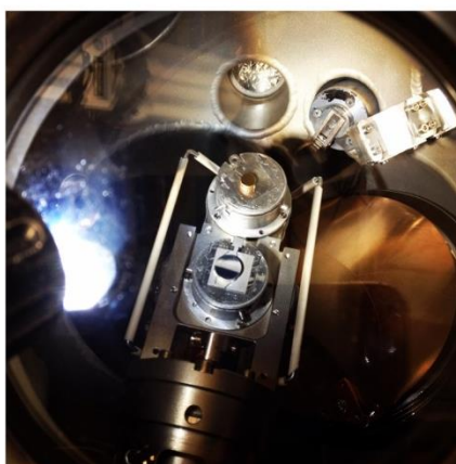
Figure 3.1 Gold and silver crystals mounted on plates in UHV.
