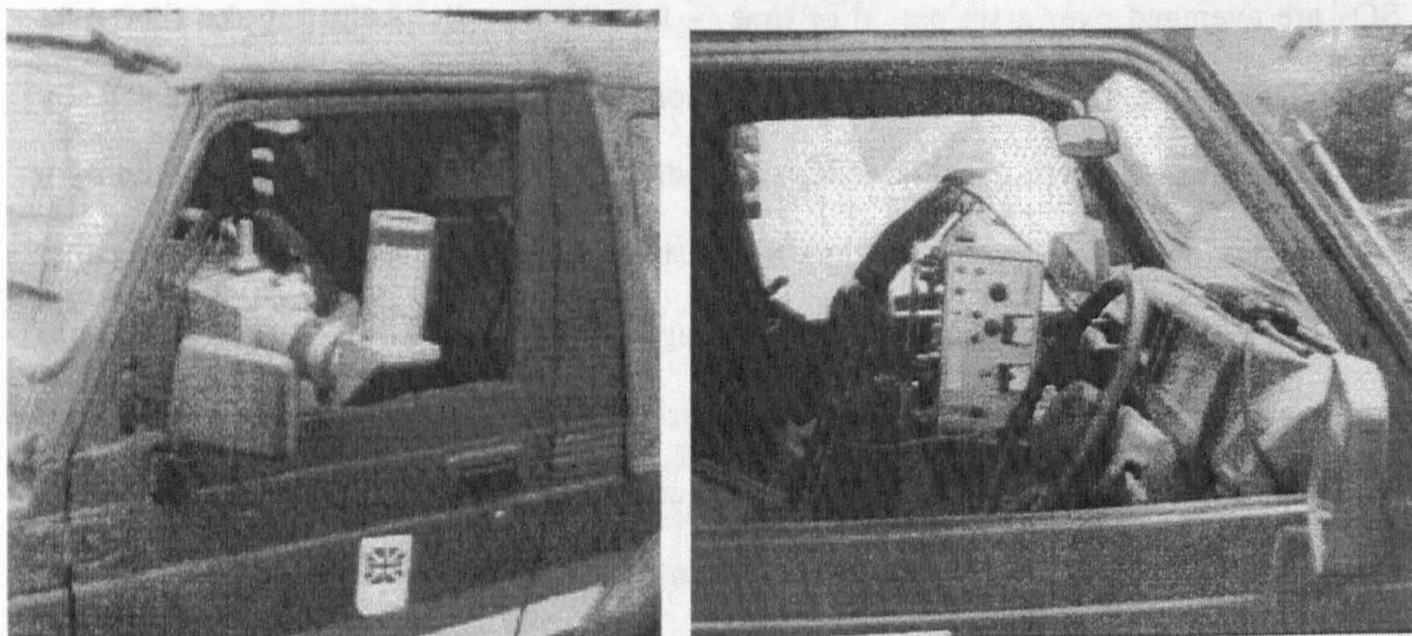
Figure 2.11. Photographs taken by the author of a COSPEC IV, owned by the University of Montreal, in operation on the Isle of Montserrat as part of the Montserrat Volcano Observatory's (MVO) monitoring effort. The vertical orientation of the right-angled telescope is essential for high quality data collection.
