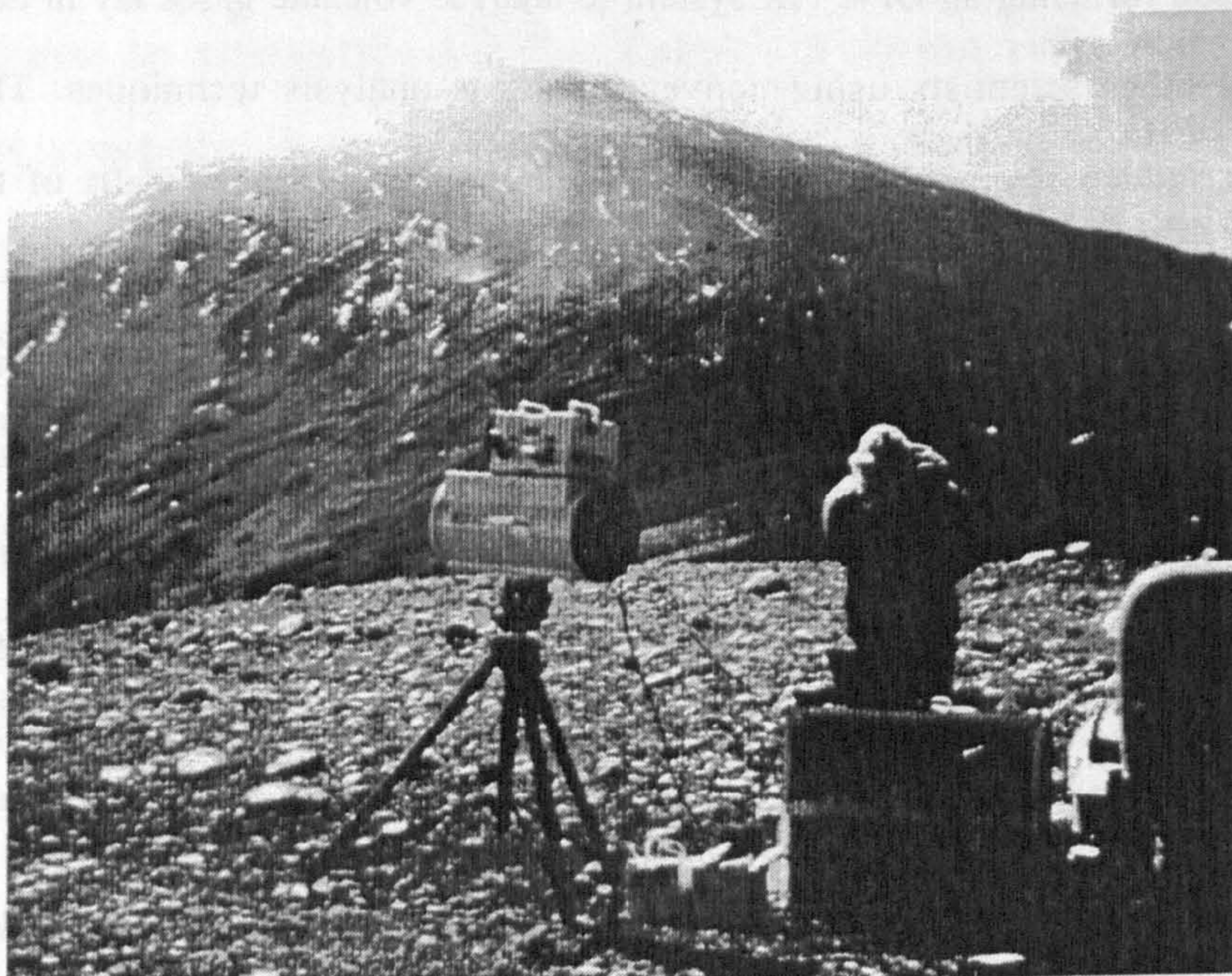
Figure 5.6. Photograph of the Midac AMS TM spectrometer being used at Pizzi Deneri below the NE Crater on Mt. Etna by C. Chaffin. The numerous tracks that cross the volcano enabled us to transport the instrument using a 4-wheel-drive Land-Rover .
