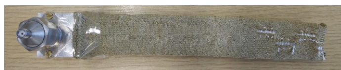
Fig.2. Slotted waveguide antenna with stitches.
