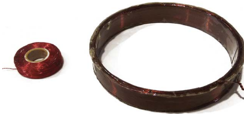
Figure 43: Coil prototypes. The small coil (left) comprises 38 layers, 43 loops per layer with an outer radius of 19 mm and height of 10 mm. The copper conductor had a diameter of 0.2 mm and conductors were spaced 0.22 mm). The big coil (right) is composed of 5 layers, 21 loops per layer with an outer radius of 60 mm and height of 18 mm. The copper conductor had a diameter of 0.8 mm and conductors were spaced 0.86 mm).
