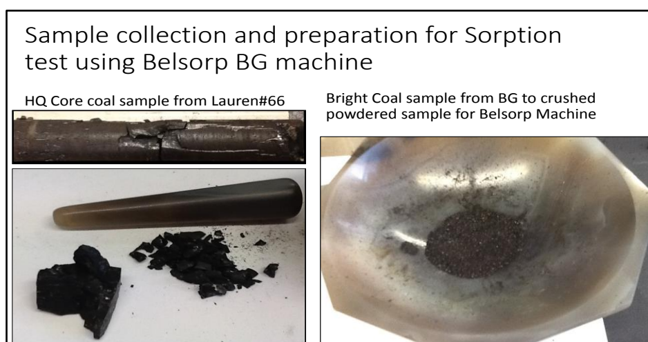
Figure 3-2 Coal powdered samples for Adsorption test using Belsorp Machine for Binary Gas Adsorption measurement
