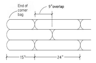
Figure 4: Earthbag wall. Source: Geiger, O. (2015, September). Earthbag Building Guide (Abridged and Adapted for Builders) – Special Edition by Osho Tapoban Publications.
