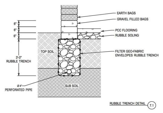
Figure 2: Rubble Trench Foundation
