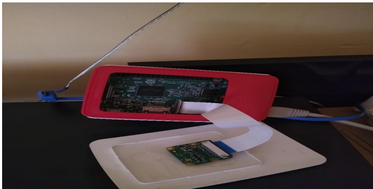
Figure A.7 The IP-based Camera Hardware Implementation
