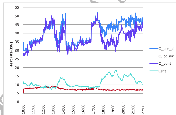
Figure 10. Evolution of thermal loads during an overload day, 19/07/2016.
